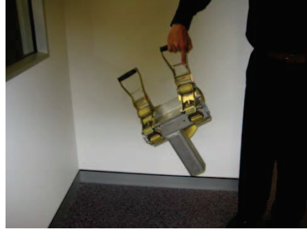
Carrying the Lifting Brackets
