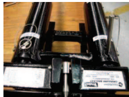
Figure 12 - Inserting Lifter Locking Pins
