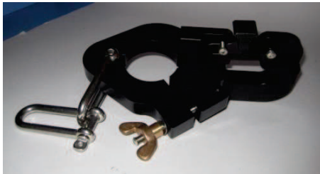
Figure 19 - Crossarm Insulator / Lifting Point / Conductor Holder
