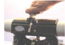
Figure 23 - Crossarm Inserted and Tightening
