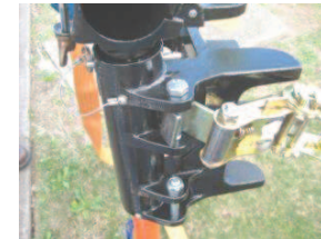
Figure 16 - Fixing Ratchet to Bracket
