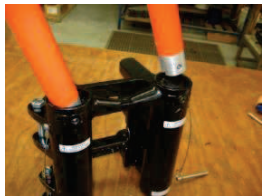
Figure 11 - Inserting Crossarm Lifter
