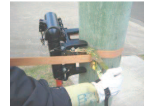
Figure 17 - Tightening Webbing Strap
