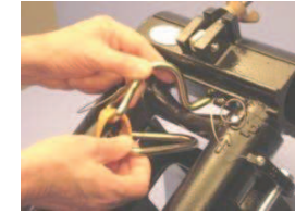
Figure 15 - Connecting Lifting Strap to Load Beam
