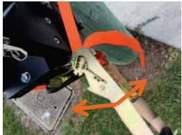
Figure 10 - Webbing Strap Tightening
